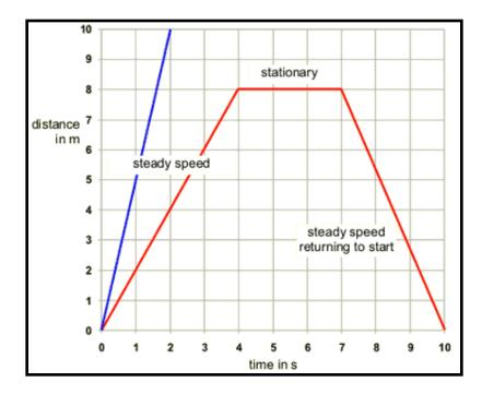
• If the line on the graph is steeper (shown by a blue line), then the speed of the object is greater.
